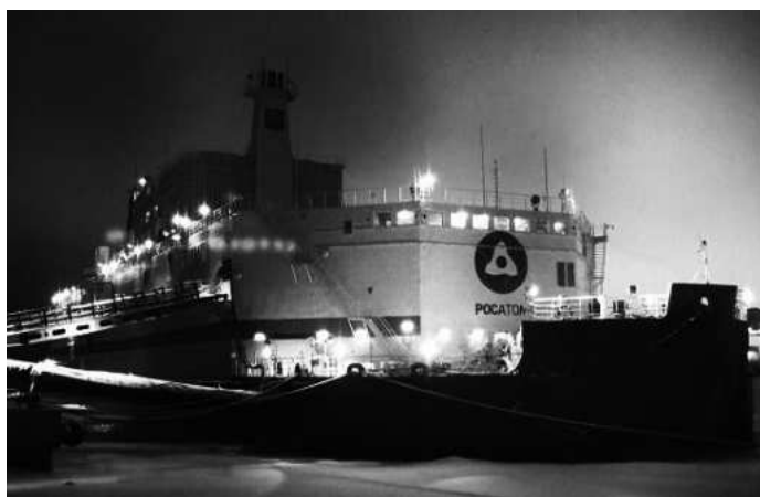
Two barge-mounted Small Modular Reactors onboard Russian vessel Akademik Lomonosov supply power to the remote arctic town of Pevek (2019).
