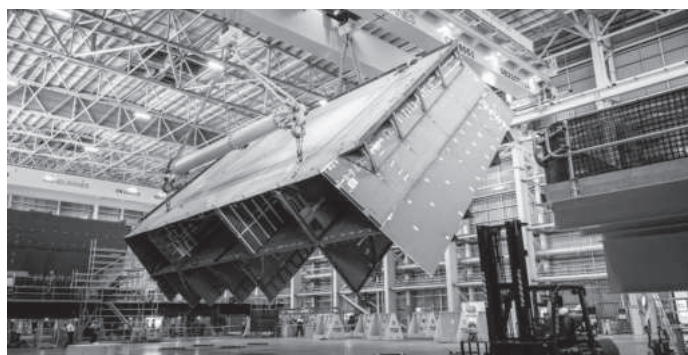
Seen here is Block 16, a prototype first 'block' for the Hunter build. It weighs in at more than 140 tonnes and involved the expertise of 35 different trades. 22 blocks go into making each Hunter class frigate. (BAE)
