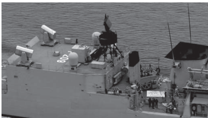
A German Type 122 class frigate illustrating its fitment of two Mk-49 21-cell RAM launchers on the aft corners of the helicopter hangar. A similar arrangement could be applied to our Hobart class AWD's increase their self-protection capability and capacity.
