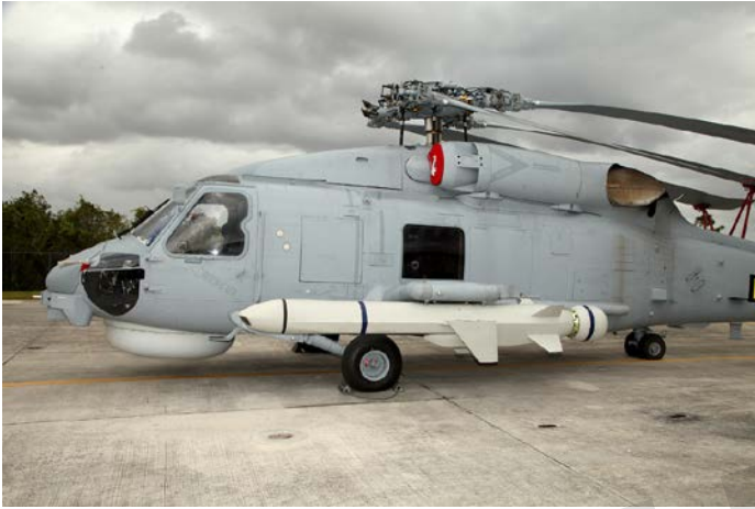
A NSM missile fitted to a Seahawk helicopter. The NSM has been certified for use from Seahawk. However, no navy that uses Seahawks and NSM has commenced the necessary integration work to certify its use. NSM from a Seahawk would extend the strike range of the RAN's fleet at sea. (Kongsberg Aust)
