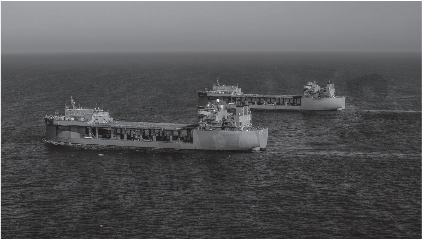
USN ESB Ships WILLIAMS and PULLER in the Gulf of Aden. The ESB ship can carry watercraft and other support elements into theatre for watercraft to range out from. However, Navy's existing LHDs can do the same. (USN)
