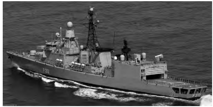
A German Type-122 class frigate with two Mk-49 RAM launchers on either beam at the aft end of her helicopter hangar roof. A similar fitment to our AWDs would give them an extra 42 anti-ASM rounds and improve their survivability to swarming attacks.
