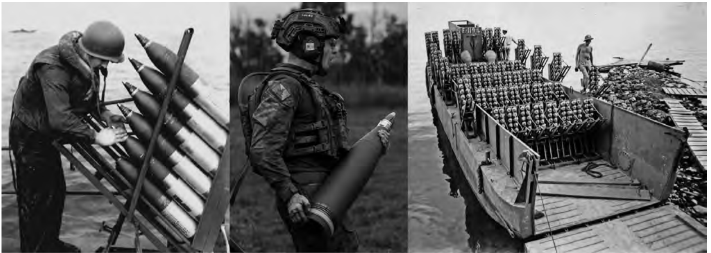
(From L to R) USN 4.5" rockets being inspected before use. They were essentially 4.5" naval shell mated to a rocket motor. (middle) An Australian Army Gunner carrying a 155mm HE round with a GPS guided course correcting fuze. (right) A USN landing ship loaded with 576 5" projectile rockets.
