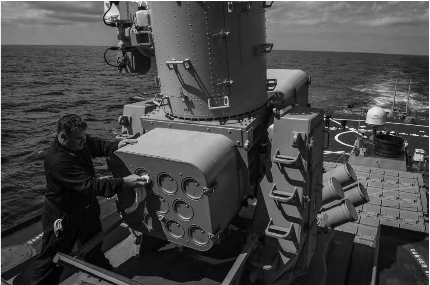
An 11 round SeaRAM on a US Navy Arleigh Burke class destroyer. Mounted on a Phalanx Block 1B in place of the 20mm gun, SeaRAM is being adopted by many navies as a step-up improvement on Phalanx. (USN)
