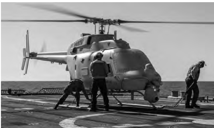
The unmanned USN MQ-8C Fire Scout can fly at 20,000ft for 15 hrs. Mounted with CEA AESA radar it could alleviate the perennial problem of attacking aircraft using the curvature of the earth to avoid giving a ship/fleet time to react to an ASM strike. It can also be used to assist with targeting the 250km ranged SM-6 anti-aircraft missile to kill the aircraft before they get into firing range. (USN)
