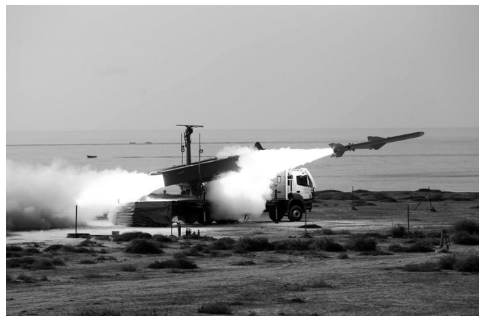
An Iranian Noor/C-802 ASM being launched from a truck. The Noor that hit INS HANIT off Lebanon does not appear to have detonated. Rather, an impact hole was left in the side of the ship and flight deck with unspent fuel causing a fire.
