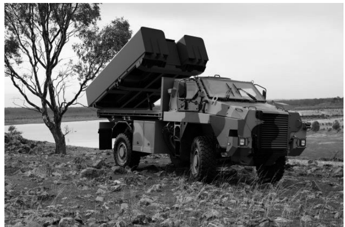
Thales Australia and Kongsberg Australia have teamed to compete for the Army's Land 4100 Ph2 contract for land based ASM capability. The concept combines the Bushmaster Ute with the NSM missile package.
