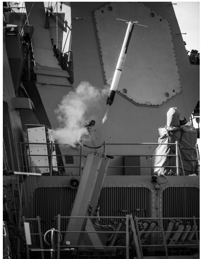
A Nulka electronic decoy round being fired. The Nulka is made in Australia and considered one of the most effective soft kill ASM decoys on the market. It was employment in 2016 by USS MASON and NITZE. (USN)
