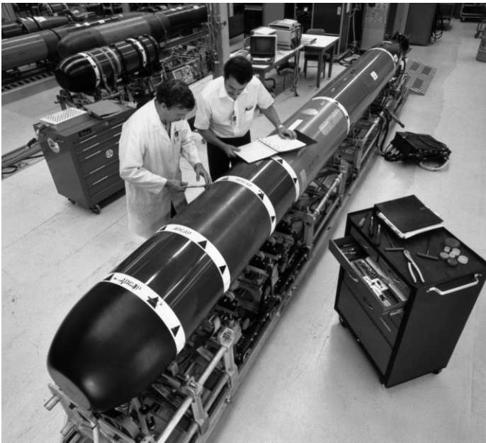
Mk 48 Mk 8 Torpedo undergoing Maintenance. The RAN is licensed to build and maintain Mk 48 torpedoes.
