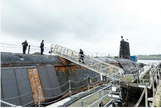
Anechoic tiles seen damaged and missing on HMS Vanguard during its second refit at Devonport in 2015 (Picture: Crown Copyright).
