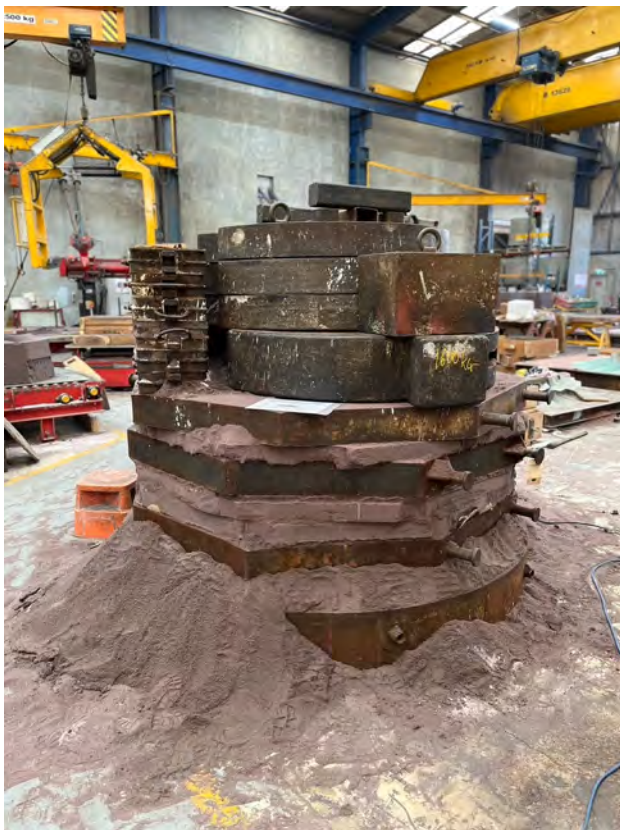
Casting of the propeller for the first stage of the memorial in the process of being cast.
