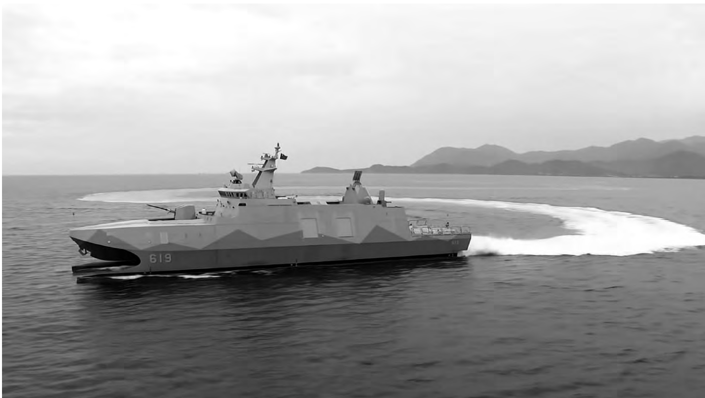
The latest Taiwanese Navy wave piercing catamaran corvette, dubbed the carrier killer, the ROCN TA CHIANG. Carrying up to 16 locally made anti-ship missiles and with a top speed of over 43kts the class of 12 will make Taiwan that little bit more difficult to topple.
