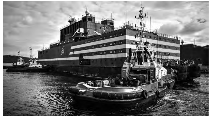
Russia's Small Nuclear Reactor Barge, built to power Russian arctic oil drills.
