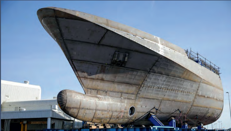
HATCH: NUSHIP ARAFURA (OPV) Two halves of the bow section joined together (Image OSBORNE Shipyard).
