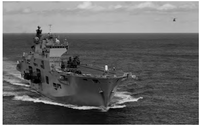
HMS OCEAN (L12) Forward CWIS Phalanx Mount - Apparently fitted on the bow to prevent a ski ramp for F-8 Harrier Use.
