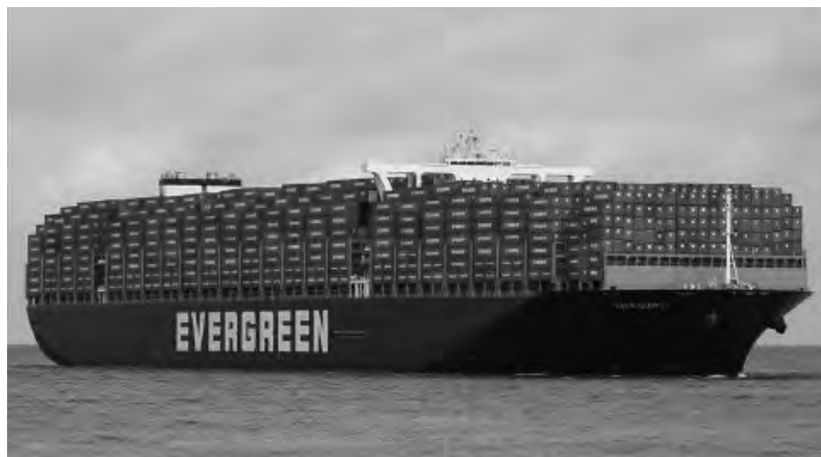
Ever Glory arriving Rotterdam Aug, 2019. Built 2019, LOA 399.98 m, Beam 58.96m, Dwt 198,937 tonnes. Image Luc van Haute Marine Traffic (MarineTraffic.com)
