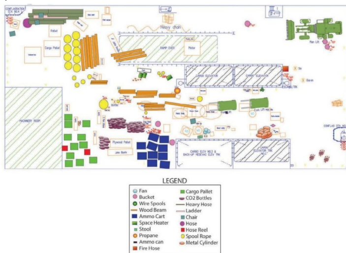
Figure 1 depicts an ATF diagram of equipment and material stored in Lower V on 12 July 2020.
