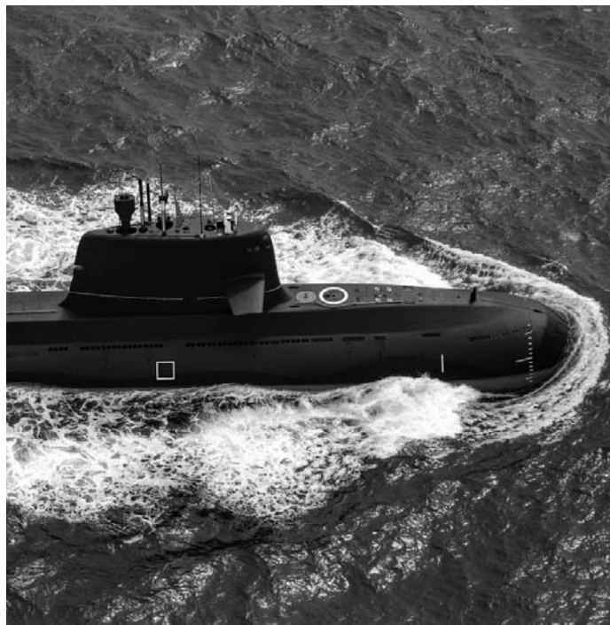
A PLA-N 3,600 tonne Yuan class diesel electric attack submarine (SSK). This is China's newest SSK which is fitted with long range anti-ship missiles and air independent propulsion. There are currently 20 of these in the water with another five building.
