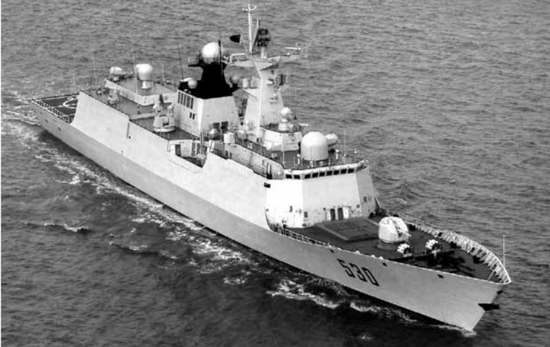
The Type 054A/Jiangkai-II class frigate XUZHOU of the East Sea Fleet. Her 32 vertically launched HQ-16 anti-air missiles have a range of nearly 50kms. Her design looks very Western with obvious stealthing techniques applied to the superstructure.
