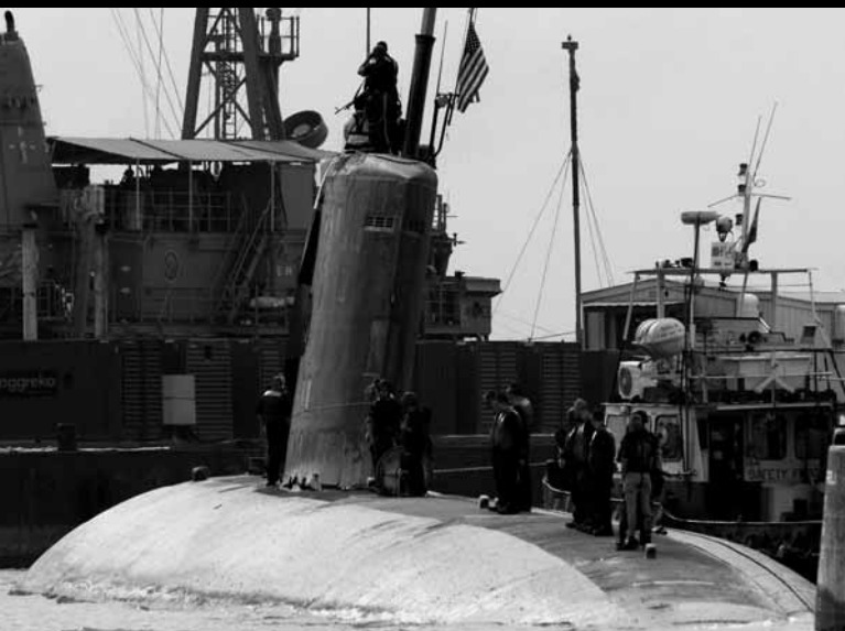
03 USS HARTFORD arrives pier side at Mina Salman pier in Bahrain for rudimentary repairs to enable her to sail, on the surface, back to the US. Notae the lean on the conning tower and ripped port side base of the tower from the collision. (USN)
