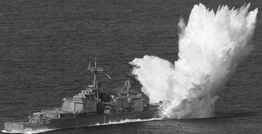
The old Spruance class destroyer ex-USS FIFE being attacked by one of two Mk-48s exploding under the bow off the US state of Washington. Wire guidance gives the submarine commander greater control on where along the ship's length his torpedoes can hit it. The second torpedo also exploded under the bow ripping it off completely from the superstructure forward. (Aug 2005, USN)
