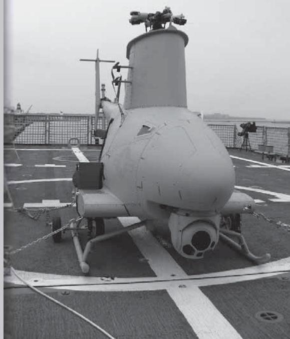
A Northrop Grumman MQ-8B Fire Scout vertical-takeoff unmanned aerial vehicle photographed recently on the flight deck of USS FREEDOM, minus its rotor blades. (USN)
