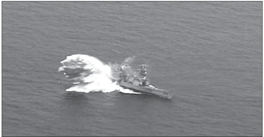
A retired Spruance class destroyer being lifted out of the water by a new Mk-48 Mod 7 exploding under the keel. (USN).
