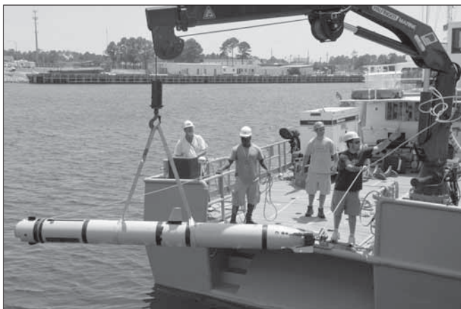
The Midsize Automated Research Vehicle (MARV) is hoisted aboard after testing. MARV is an experimental platform supporting the USN's planned unmanned underwater vehicles (UUV) in particular the 21 inch (533mm) torpedo sized Heavy Weight Vehicle (HWV). Missions for the HWV will include clandestine anti-mine and tactical reconnaissance, littoral access oceanography and long endurance submarine decoy. (USN)
