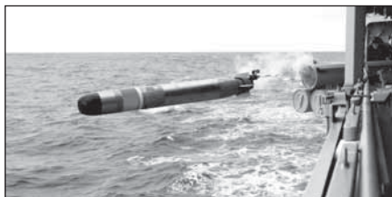
A test MU90 Torpedo being fired from the Anzac class frigate HMAS TOOWOOMBA during last June. When finally integrated into the ADF, the MU90 will provide a potent ASW weapon against submarines in shallow water. (RAN)
