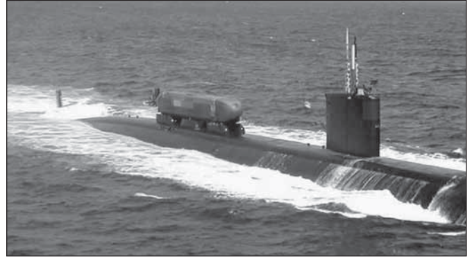
Lithium-Ion batteries are used for the USN's Advanced SEAL Delivery System (ASDS) seen here piggy backing off the SSN USS GREENVILLE. Li-ion batteries offer significantly higher power densities over Lead-Acid batteries and are rugged enough for fleet service. (USN)
