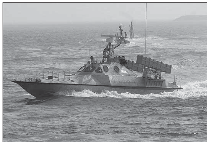
An IRG high speed missile boat fitted with two Chinese made C-701 anti-ship missiles. The C-701 is unique as it has a millimetre wave radar which is undetectable to many warships such as the Anzac class.
