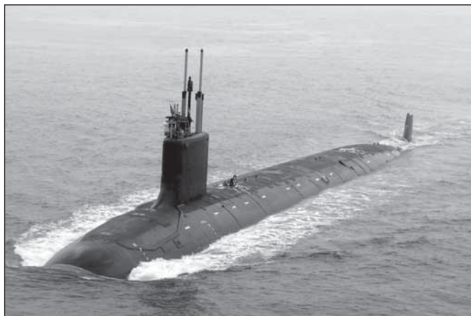
The Virginia class SSN USS VIRGINIA on the surface during her initial sea trials. With the advance of technology in the form of battery life, stored energy and electric motor power the RAN could potentially use the existing Virginia design for a conventional submarine class. (USN)
