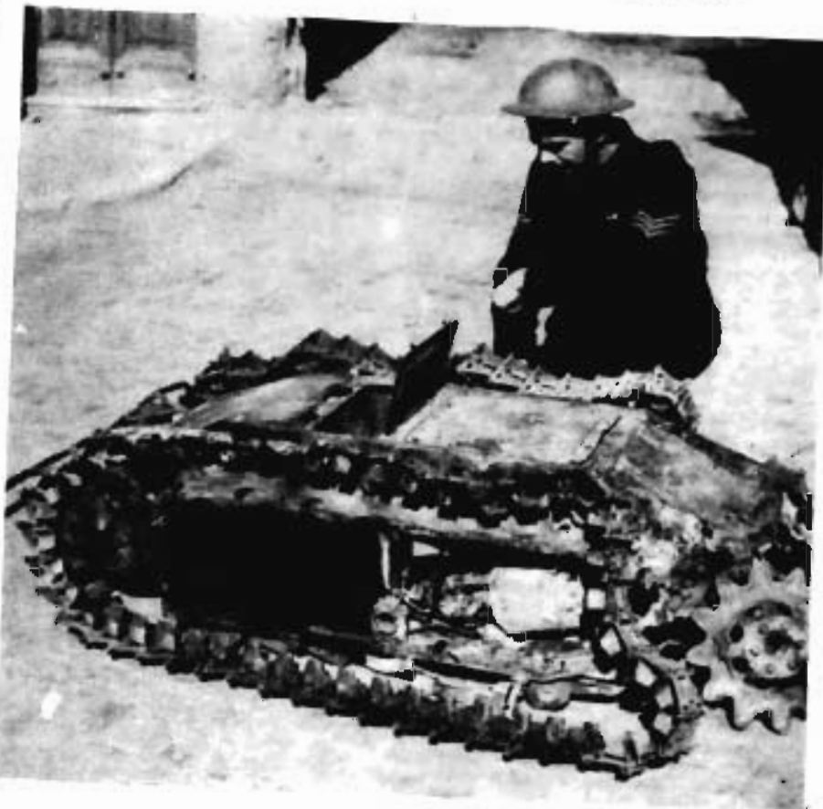
One of the Nazi tanks, called "doodlebugs" by the Allied troops, used unsuccessfully by the Germans at Anzio beachhead and later at Cisterna. Originally thought to be radio-controlled, this captured "doodlebug" revealed the electric cable by which it was steered. The "doodlebugs" contain 250 lb. of explosives and are 69 inches long.—Courtesy "Herald."
