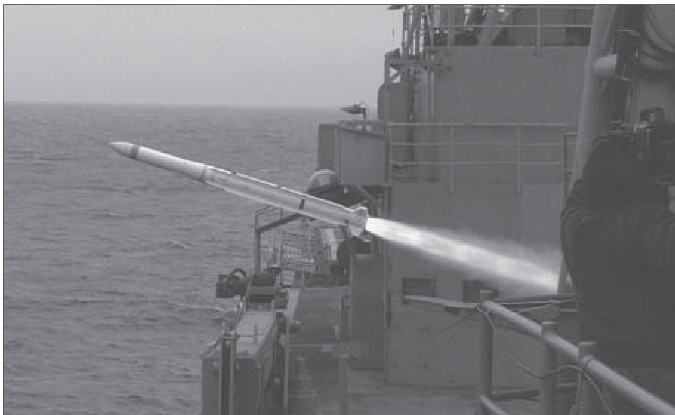
An ESSM in flight. The new ESSM has the same guidance section as the older Sea Sparrow but with a new propulsion unit, flight control surfaces and mid course guidance. (Raytheon)
