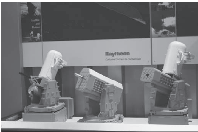
Models of Raytheon's Close In Weapon System solution. (From L to R) The Phalanx Block 1B with larger magazine, higher rate of fire, longer range, more accurate aiming systems and with TV/IR back up. The RAM launcher for the fire and forget short range missile for defence against anti-ship missiles. Finally, the combination for the Phalanx Block 1B and the RAM launcher to form the Sea RAM, a bolt to the deck fully autonomous ship self defence weapon system.
