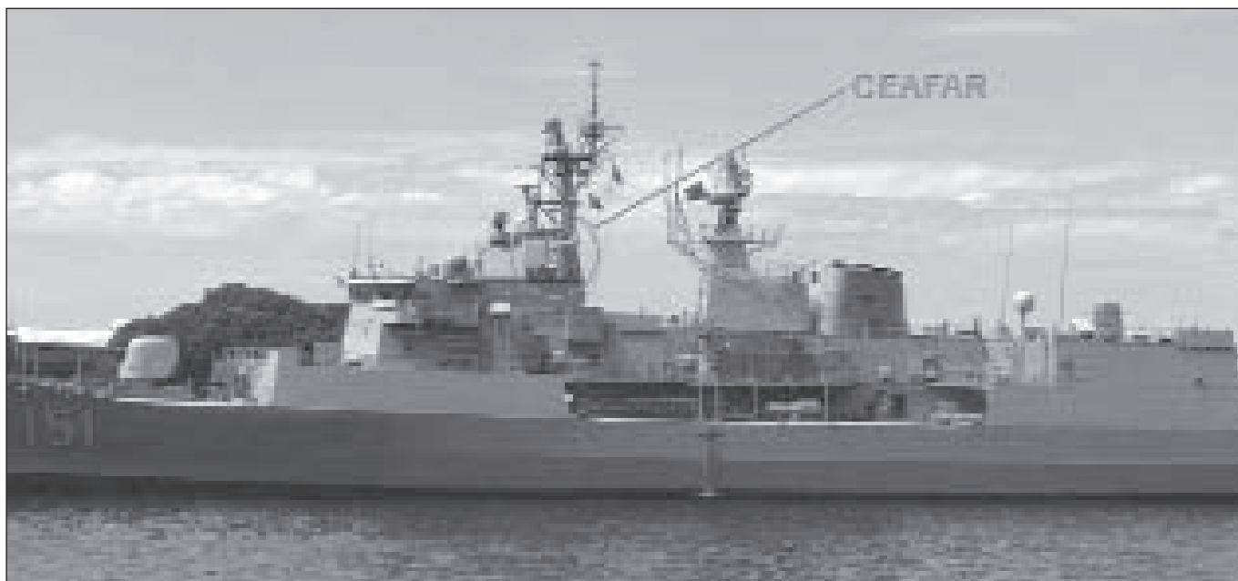
The sea trials test ship for the CEA-FAR radar was HMAS ARUNTA. A temporary fit of two of the passed array panels for the first at-sea trials can be seen in this image. The radars and their integration into the 9LV combat system performed well. (RAN)
