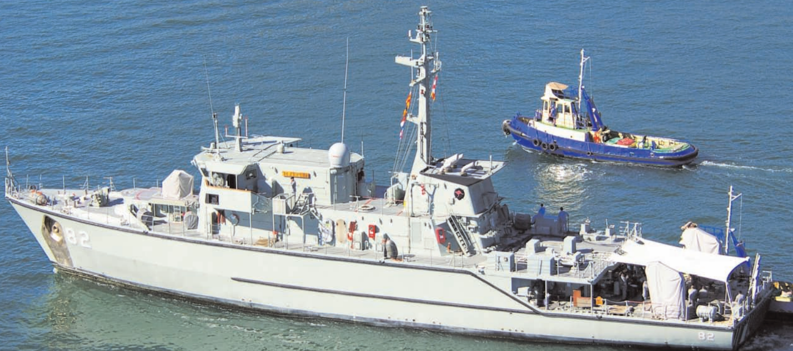
HMAS HUON being towed to Garden Island in Sydney for storage. Note most of her mine hunting equipment, radars, life rafts, anchor etc have been removed. Two of the Huon class minehunters are being placed into storage due to manpower shortages, cost savings and to the perceived strategic environment not requiring six RAN mine hunters. (Chris Sattler)
