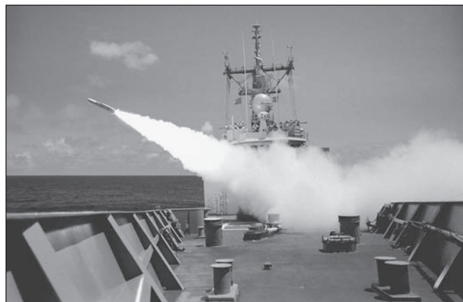
HMAS ADELAIDE 'lets fly' with a Standard SM-1MR anti-aircraft missile. While ADELAIDE and CANBERRA will be decommissioned early their four sister ships will be upgraded with Standard SM-2MR as the current batch of SM-1MR missiles have reached the end of their service life, and the fact that new missiles are impossible to obtain. (RAN)
