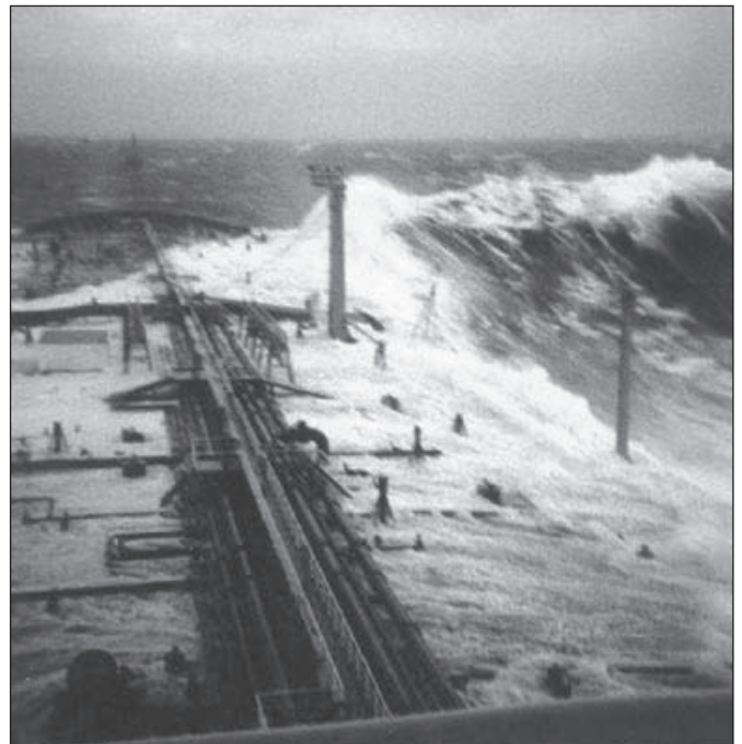
This rare photo of a rogue wave was taken by first mate Philippe Lijour aboard the supertanker ESSO LANGUEDOC during a storm off Durban in South Africa in 1980. The mast seen to starboard in the photo stands 25 m above mean sea level. The wave approached the ship from behind before breaking over the deck, but in this case caused only minor damage.
