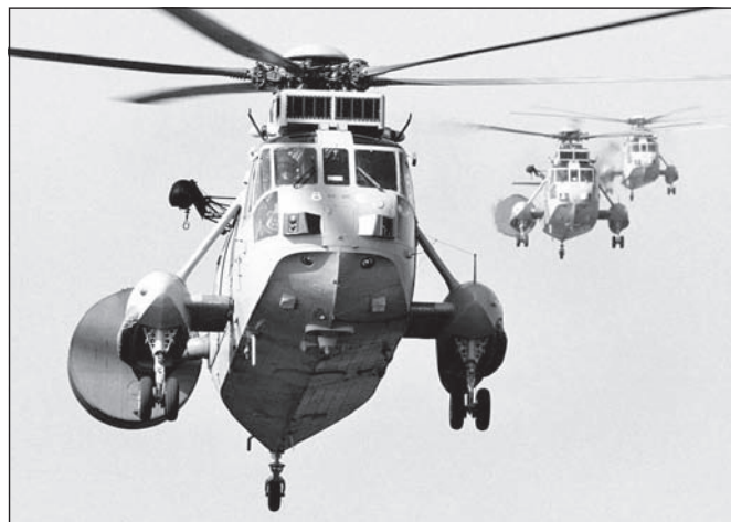
Four Sea King Mk-7 were deployed to Operation Iraqi Freedom onboard HMS ARK ROYAL. The new radar and processing technology made it possible for the Mk-7 to track moving land targets and downlink this information to ground commanders via Link 16. (RN)
