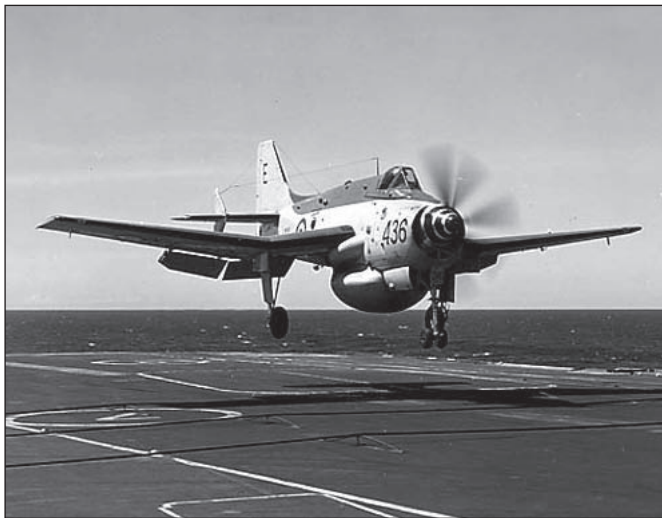
A RN Gannet AEW aircraft about to 'trap' aboard a RN aircraft carrier. The Gannet was fitted with an AN/APS-20F radar which could detect a destroyer sized target at over 200 miles. It had one pilot and two observers and a data link back to the carrier. (RN)
