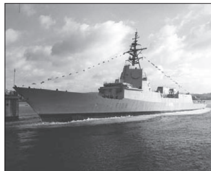
The Spanish Navy frigate MÉNDEZ NÚÑEZ, fourth and last of the F-100 class, being launched at the Izar Shipyard in Ferrol, Spain. The ship was launched 80% complete. (Izar)
