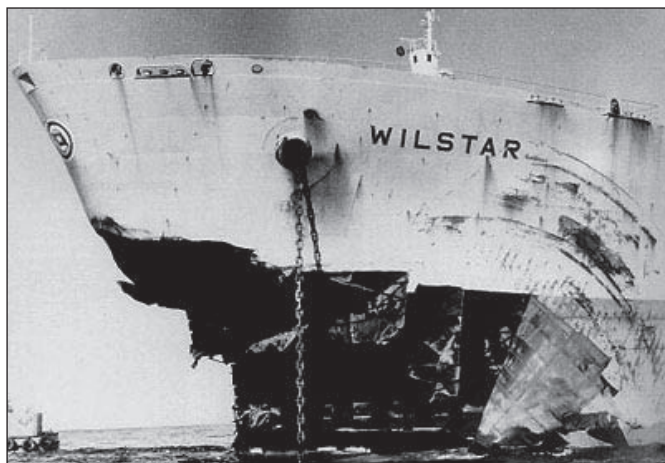
Rogue waves are most common in the Agulhas current off the east coast of South Africa, with numerous well documented cases of extreme individual waves, including some striking photographs of damaged ships. This bow damage was received by the Norwegian tanker WILSTAR in 1974. (Photo DLR)
