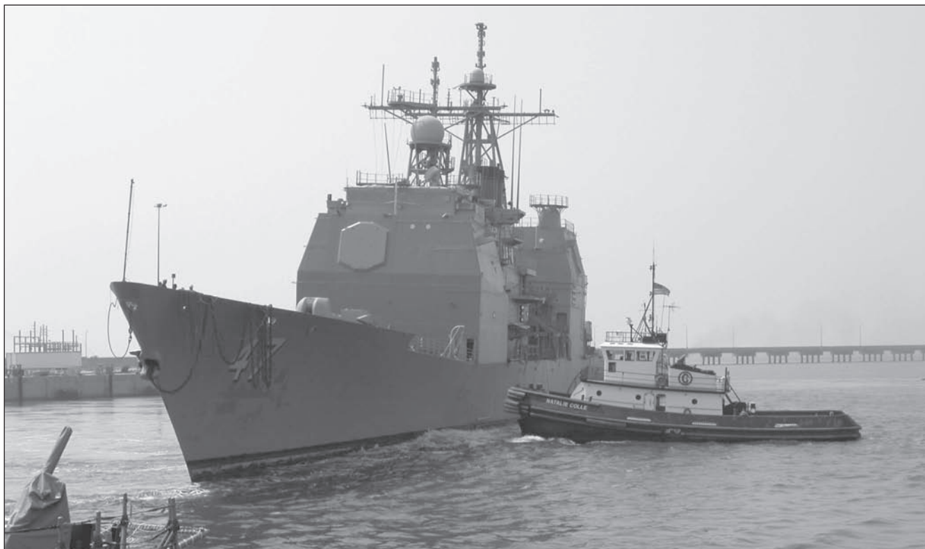
The last passage. The former USS TICONDEROGA is towed from her decommissioning berth at Pascagoula, Mississippi, for the inactive storage yard at Philadelphia. She was first commissioned on 22 January 1983. Note the absence of the main mast radar, fire control radars, Phalanx and the covered up bridge windows. At one stage there was a very real offer to have 2-3 of the first baseline lot of the Ticonderoga class (5 ships worth) leased to the RAN to avoid their early retirement from naval service. To any navy outside of the US these early Ticonderoga class cruisers still represent a quantum leap in capability. (USN)
