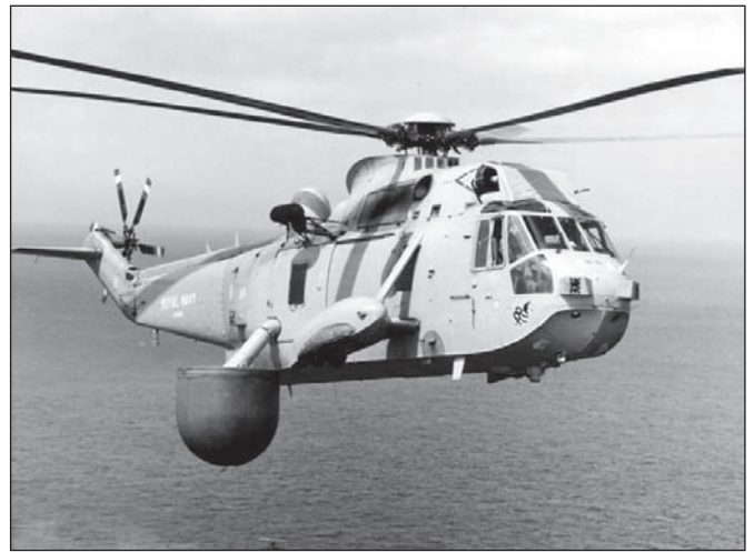
The AEW Sea King was developed over an 11 week period when it became painfully obvious during the 1982 Falklands conflict that AEW was still a necessity. Two Sea Kings fitted with a searchwater radar deployed to the Falklands for the first time on HMS ILLUSTRIOUS when she relieved HMS INVINCIBLE after the conflict. (RN)
