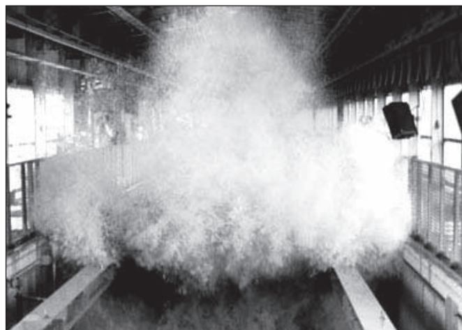
A giant wave produced with a hydraulically-powered wave generator in the Giant Wave Tank in Hanover in 2002. As part of the ‘MaxWave’ project, a team at the Technical University of Berlin worked on simulating their production. Their work guided by computer modelling, the team found rogue waves appear to be formed when slow-moving waves are caught up by a succession of faster waves moving at more than twice their speed, then merge together. (Technical University of Berlin)
