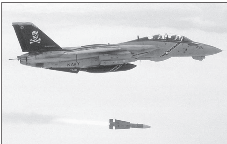
A USN F-14 Tomcat firing an AIM-54 Phoenix AAM. The US Navy retired the AIM-54 Phoenix long-range air-to-air missile on 30 September 2004 after 30 years of service. The Phoenix had a range of 180kms. It was the first radar-guided missile that could be launched in multiple numbers from the same aircraft simultaneously against different targets. (USN)
