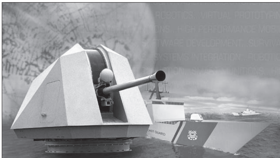
The new Mk-110 57mm CIGS for the new DD(X). Depicted is the original version known as the Bofors Mk-3 which will arm the US Coast Guard's new ships.
