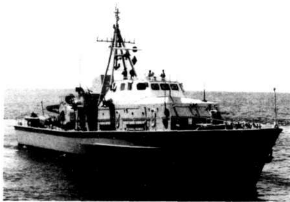
The four River class coastal minehunters, which entered service in 1981, are propelled by two non-magnetic Voith Schneider vertical axis propulsion units which are designed to provide excellent manoeuvrability and quietness of operation. Pictured here is SAS UNKOMAAS
