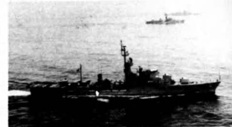
FERRE after second reconstruction. Note the four twin launchers for the Exocet surface to surface missile system, immediately forward of "X" turret. Since this photograph was taken "X" turret has been removed to provide a larger helicopter deck, the bridge enclosed, the after funnel remodelled and the two 40mm anti-aircraft guns replaced by twin 40mm Breda-Bofors 1.70 compact. FERRE was formerly the British Daring class destroyer HMS DECOY, purchased in 1969
