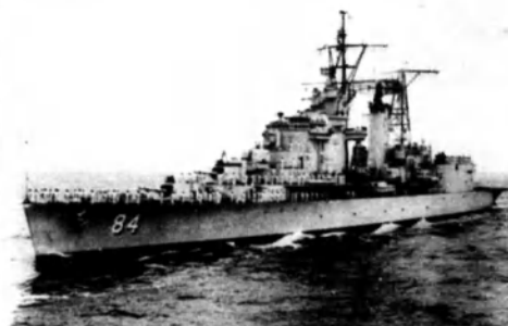
AGUIRRE, ex Dutch DE ZEVEN PROVINCIE, was completed in 1953 and sold to Peru in August, 1976. Following the sale she was rebuilt into a helicopter cruiser with space for three Sea Kings. The conversion was completed in the USA in October, 1977
