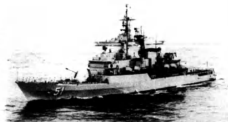
Only a recent addition to the fleet (1978) MELITON CARVAJAL is a "modified Italian Lupo" class frigate. The massive gun forward of the bridge is a single 5 inch 54 calibre mount. Two 40mm 70 twin compact guns are also carried, as well as four twin Otomat SSMs, one Albatross/Aspede octuple A/A missile launcher, two 20 barrelled rocket launchers, two twin Mk32 A/S torpedo tubes and one helicopter. A small but very capable ship!
