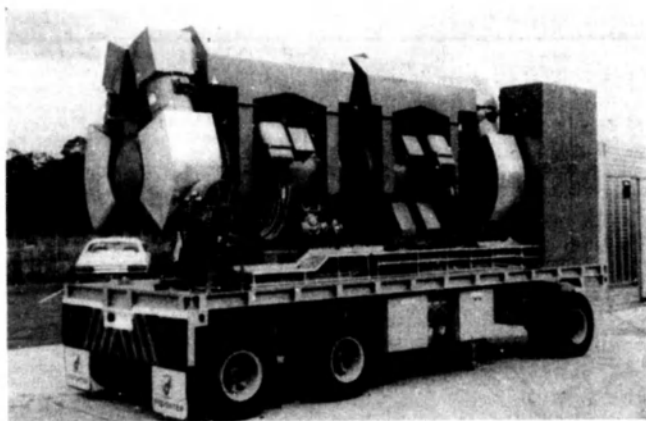
Mobile frequency changer (with canopy removed), designed by the Power Systems Department of GEC Project Division
