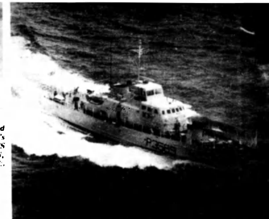
One of four new patrol craft, HMNZS ROTUITI was built by Brooke Marine and completed in 1975. She carries one twin 50 calibre machine gun forward of the bridge, and one combination 81 mm mortar 50 calibre machine gun aft, plus numerous small arms. The craft have not proved a great success operationally and with limited funds available to the Navy, will need to see out many more years of service. (Photo — Royal New Zealand Navy).
