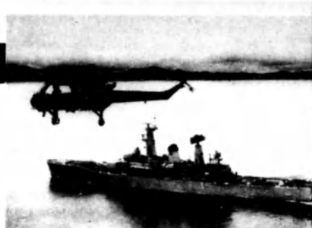
HMNZS WAIKATO, shown here with her Wasp helicopter airborne, has been in commission since 1966. She retains her anti-submarine mortar in the well aft, but mounts no torpedoes. (Photo — Royal New Zealand Navy).
