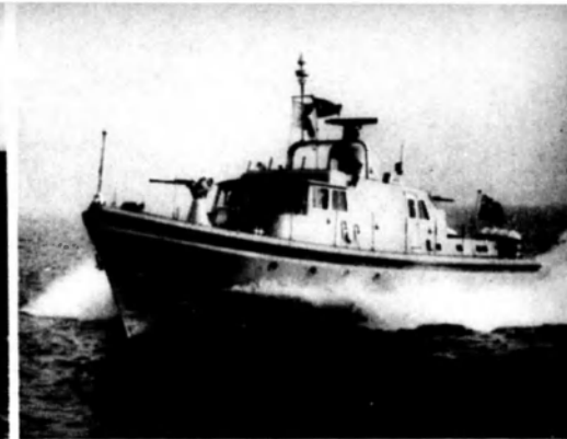
The R.L.N.S. SUSAN, the first of three gas-turbine fast patrol boats designed and built by Vosper Thornycroft for the Royal Libyan Navy. She is seen discharging one of her Nord-Aviation wire-guided missiles.
