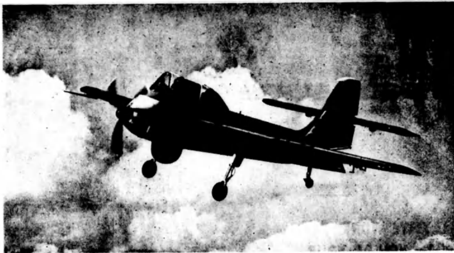
The Short Seamew, powered by an Armstrong-Siddeley Mamba turbo-prop engine, in flight. It carries the latest radar "search and strike" equipment. The radar scanner is housed in the bulge under the cockpit.
