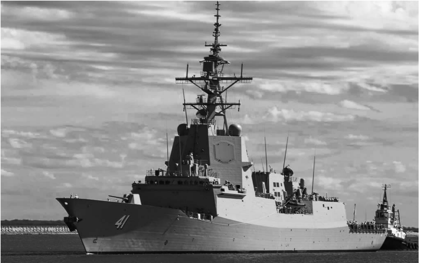
NUSHIP BRISBANE (D41) - CODOG (using less powerful Gas Turbines) is already fitted in many global frigate solutions and the AWD Hobart class destroyers.
