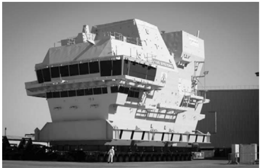
HMS PRINCE OF WALES (R09) Forward Island Bridge Module
