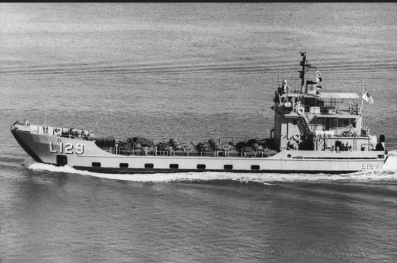
HMAS TARAKAN with a full load of 12 M-113 APCs and one 5-ton Mack truck. The LCH's had a very good load carrying capacity. (RAN)
