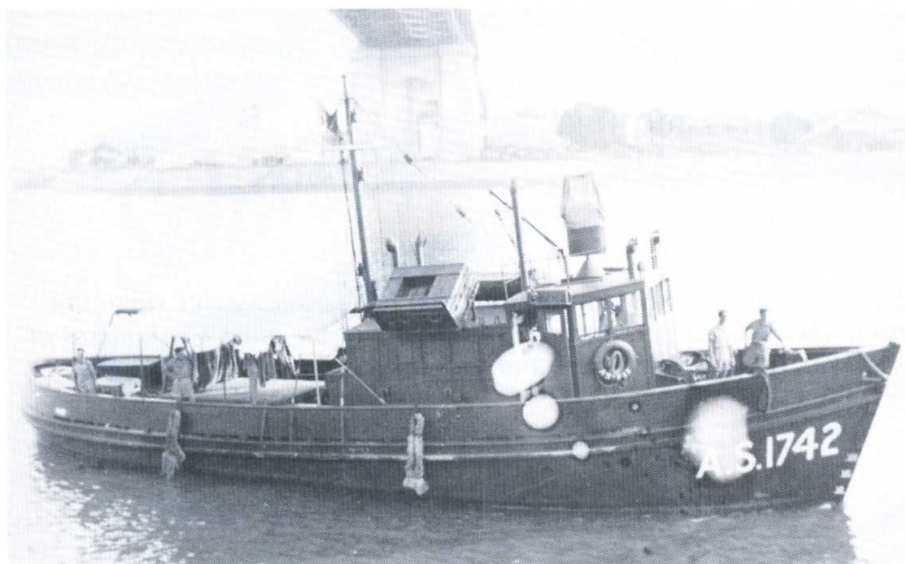
The "66 foot Wooden Cargo Vessel", AS1742 MADALYA under Storey Bridge on the Brisbane River. As comparison with AS25 shows, she was built to a typical seine trawler design of the 1940s.
